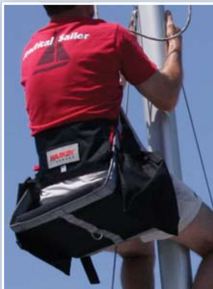
Comfortable and secure, the Brion Toss harness (above left) is based on a rescue harness design. The Harken chair (above center) had the largest seat platform and deepest cushion with side pockets. The Topclimber (at right) was the only device that allowed the user to ascend solo.
